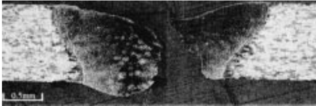
Fig. 16 Tensile fracture of AA6111 twb
